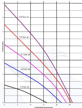
Flow rate and pressure vary depending on the air sent to the pump:
